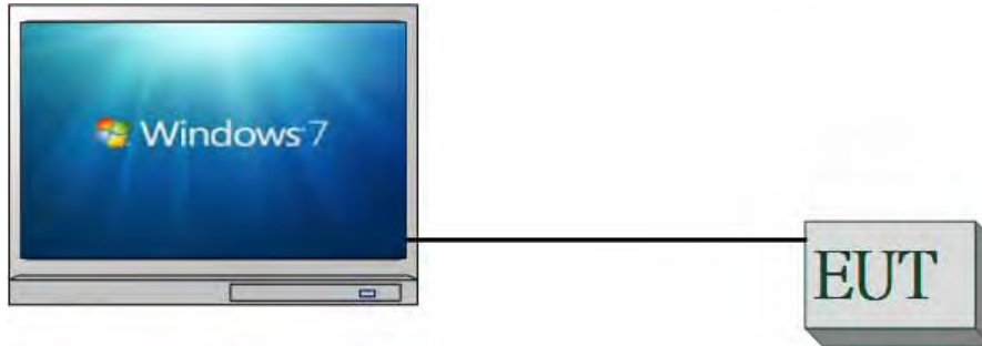
Fig. 2-2 AC Power Line Conducted Emission Configuration
