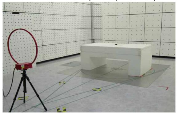
Radiated Emission Set up Photos (Below 1GHz)
