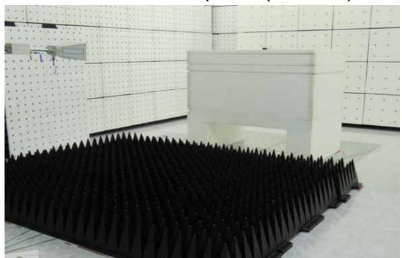
Radiated Emission Set up Photos (Front View)
