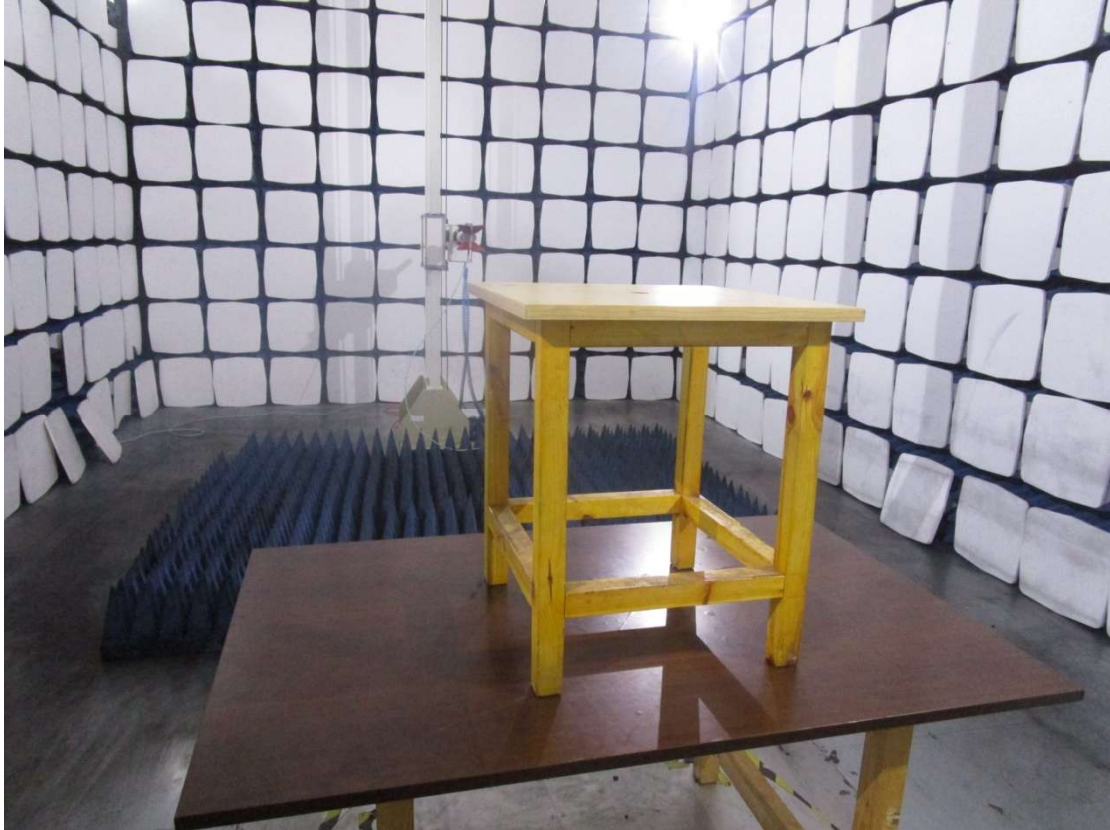
1.5M-Height Turntable Test Table (Close-Up Shot shows the height of the table without EUT)
