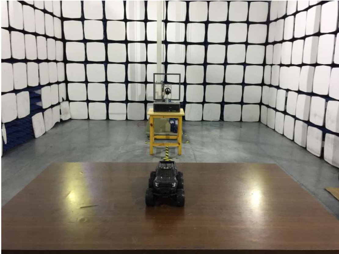
Radiated Emission Test Setup (9 kHz to 30 MHz) from 0.8M-Height Turntable Test Table
