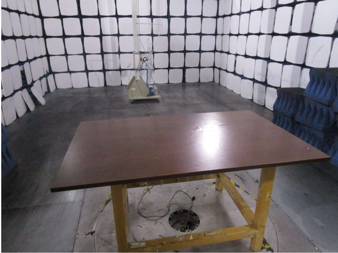
0.8M-Height Turntable Test Table (Close-Up Shot shows the height of the table without EUT)
