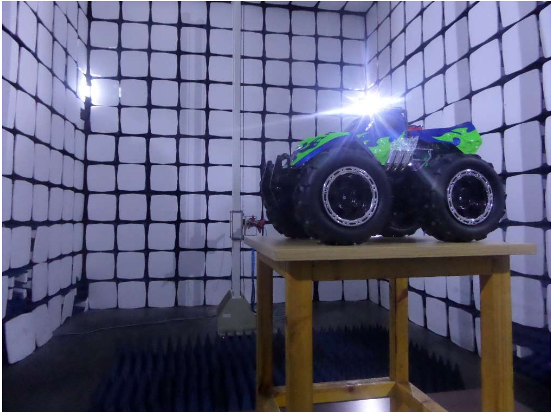
Radiated Emission Test Setup (above 1 GHz) from 1.5M-Height Turntable Test Table
