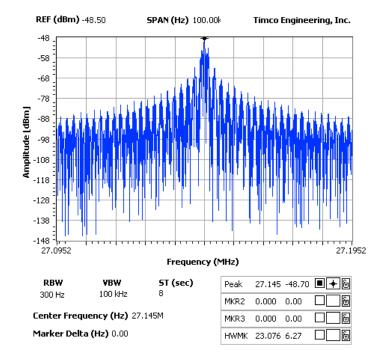
${\tt METHOD}$  OF <code>MEASUREMENT:</code> A small sample of the transmitter output was fed into the spectrum analyzer and the attached plot was taken. The vertical scale is set to 10 dB per division.
