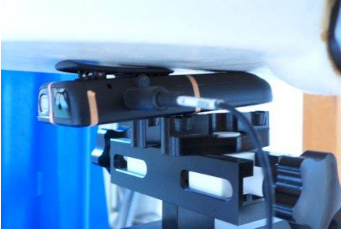
Pic. 9: Test position back side of EUT towards the phantom, 0 mm gap, belt clip and headset attached.
