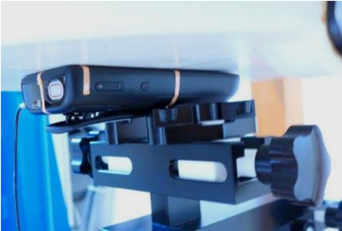
Pic. 8: Test position front side of EUT towards the phantom, 0 mm gap, belt clip and headset attached.
