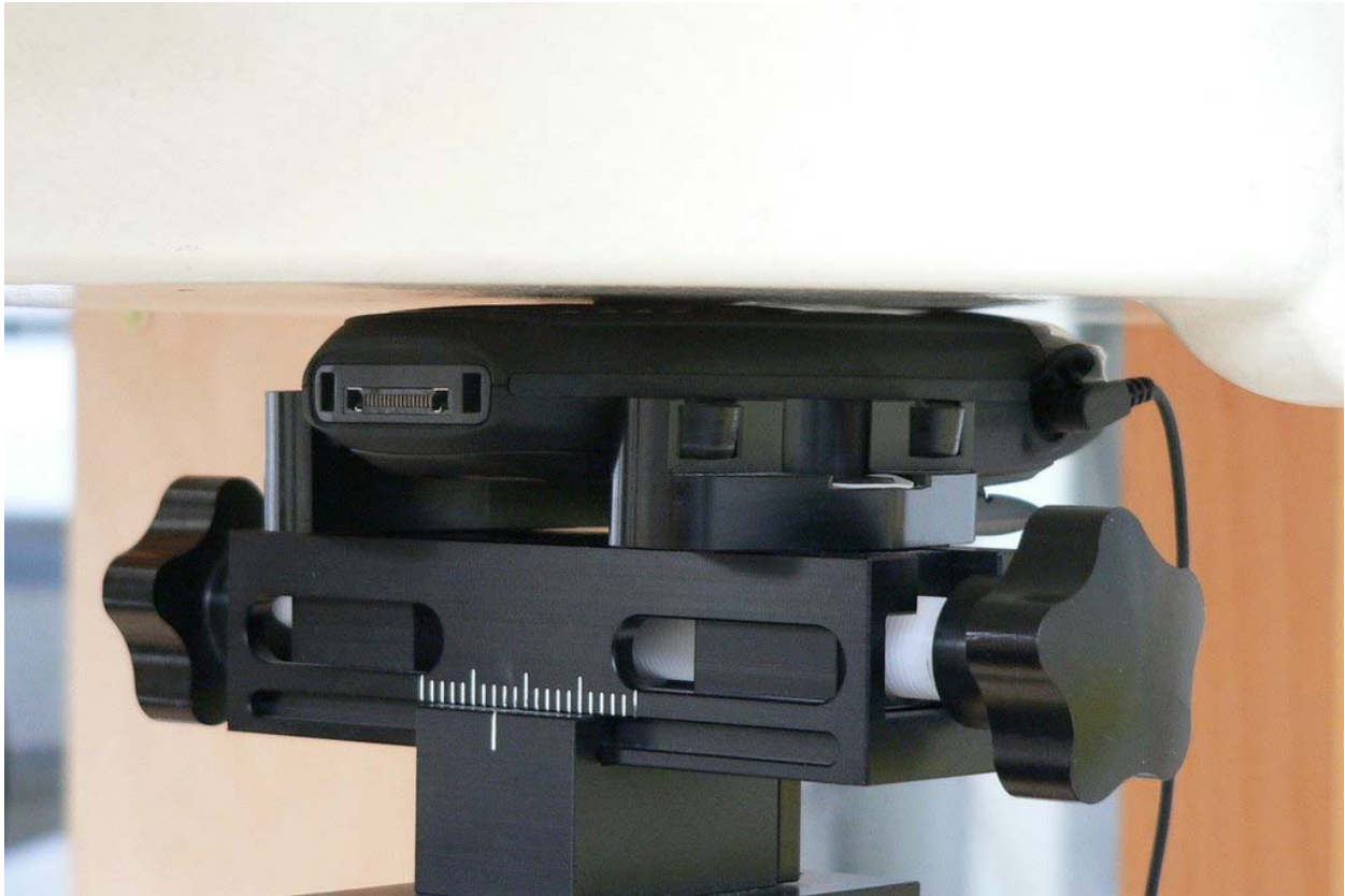
Fig. 41: Bottom view of body worn, HS connected, display up (towards the phantom).
