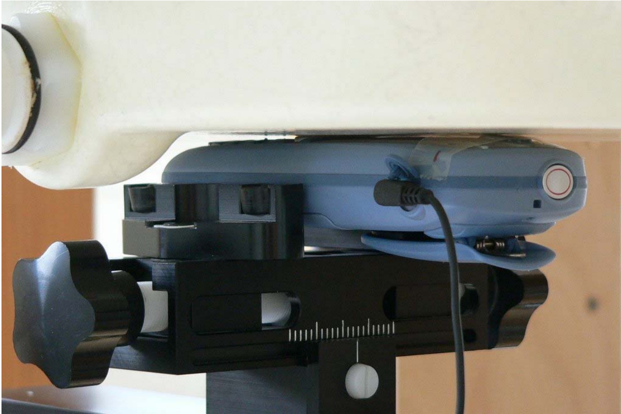
Fig. 42: Top view of body worn, HS connected, display up (towards the phantom).
