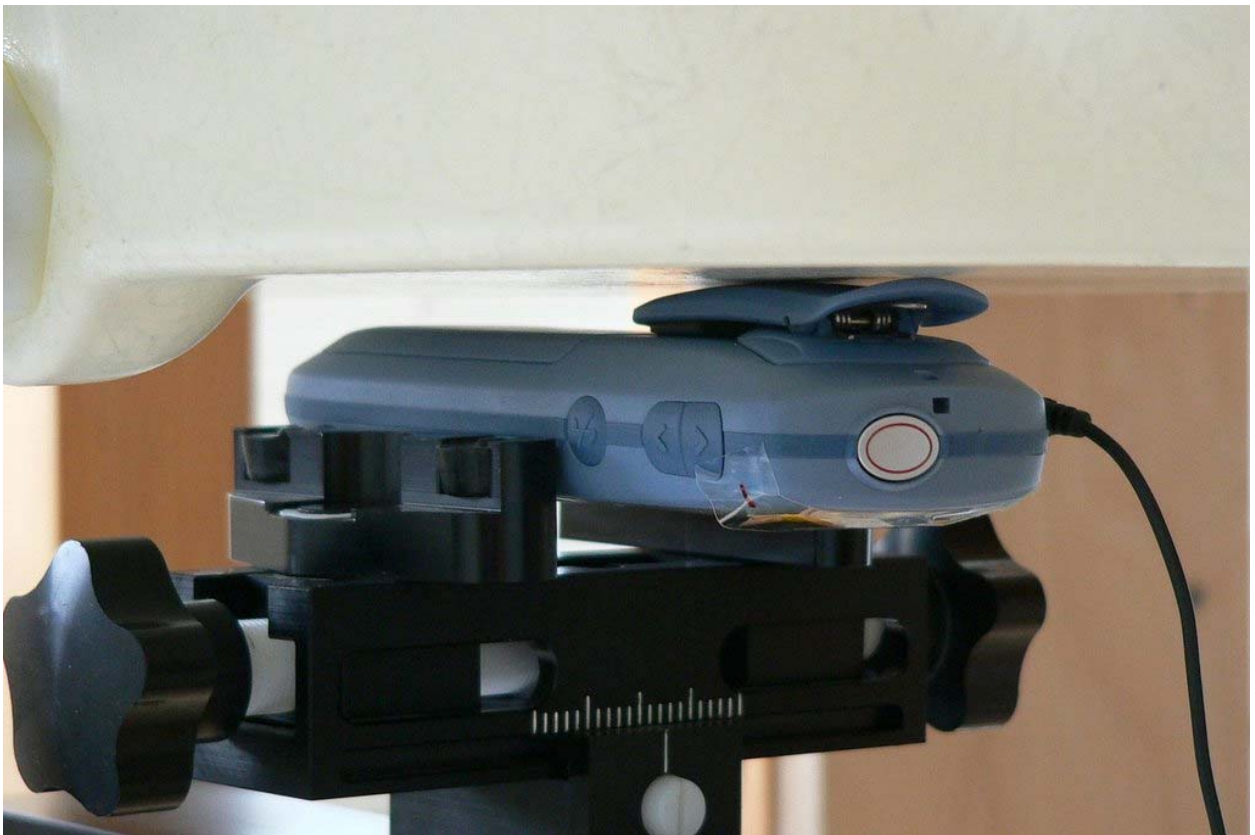
Fig. 44: Top view of body worn, HS connected, display down (towards the ground).
