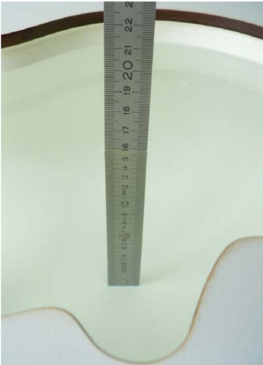
Fig. 45: Liquid depth for IEEE 802.11 b/n Head measurements
