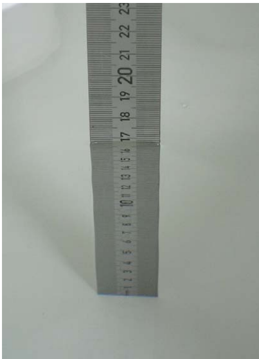
Fig. 47: Liquid depth for IEEE 802.11 b/n Body measurements
