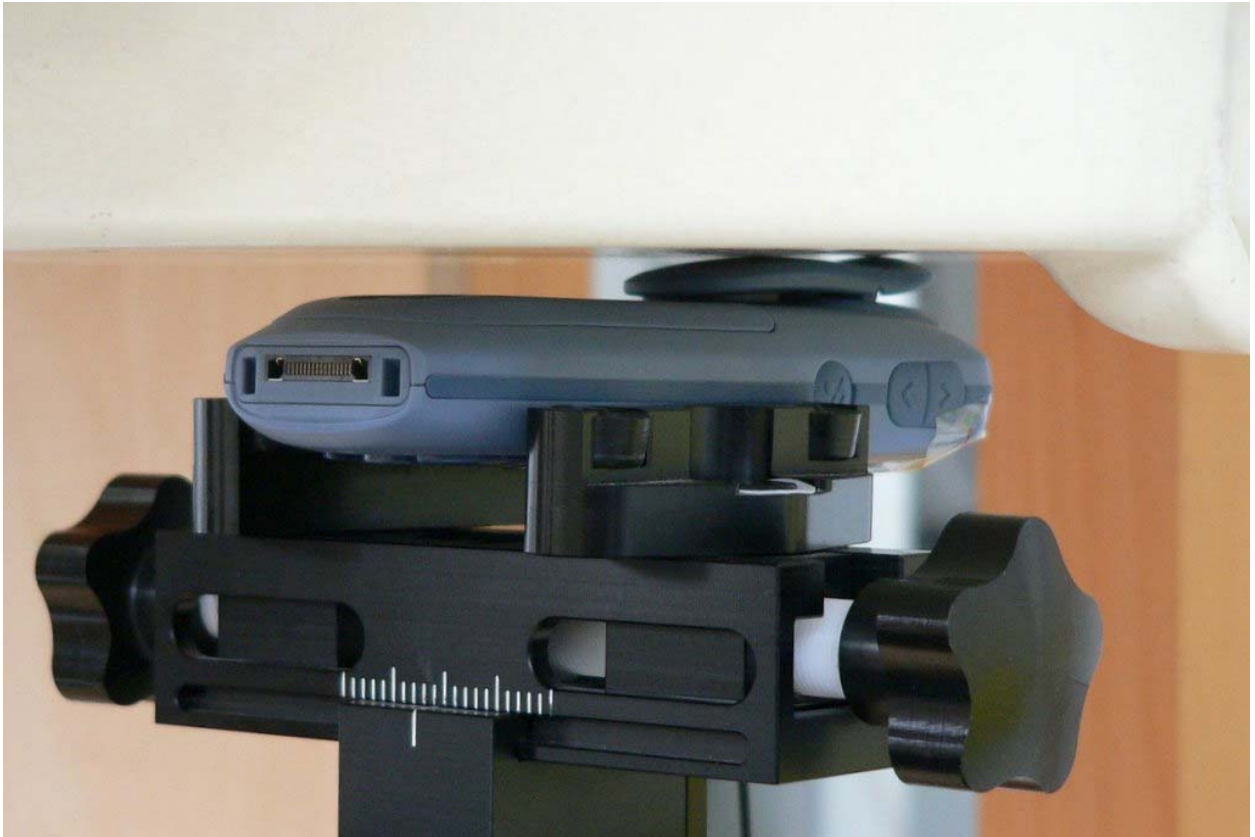
Fig. 43: Bottom view of body worn, HS connected, display down (towards the ground).
