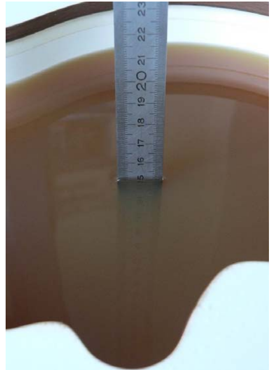
Fig. 46: Liquid depth for IEEE 802.11 a/n Head measurements
