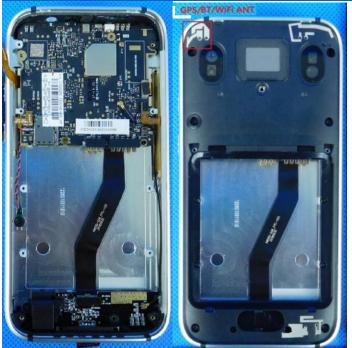
Antennas in the right picture are re-used as DECT antennas, not changed. Bottom PCB in not changed at all.
