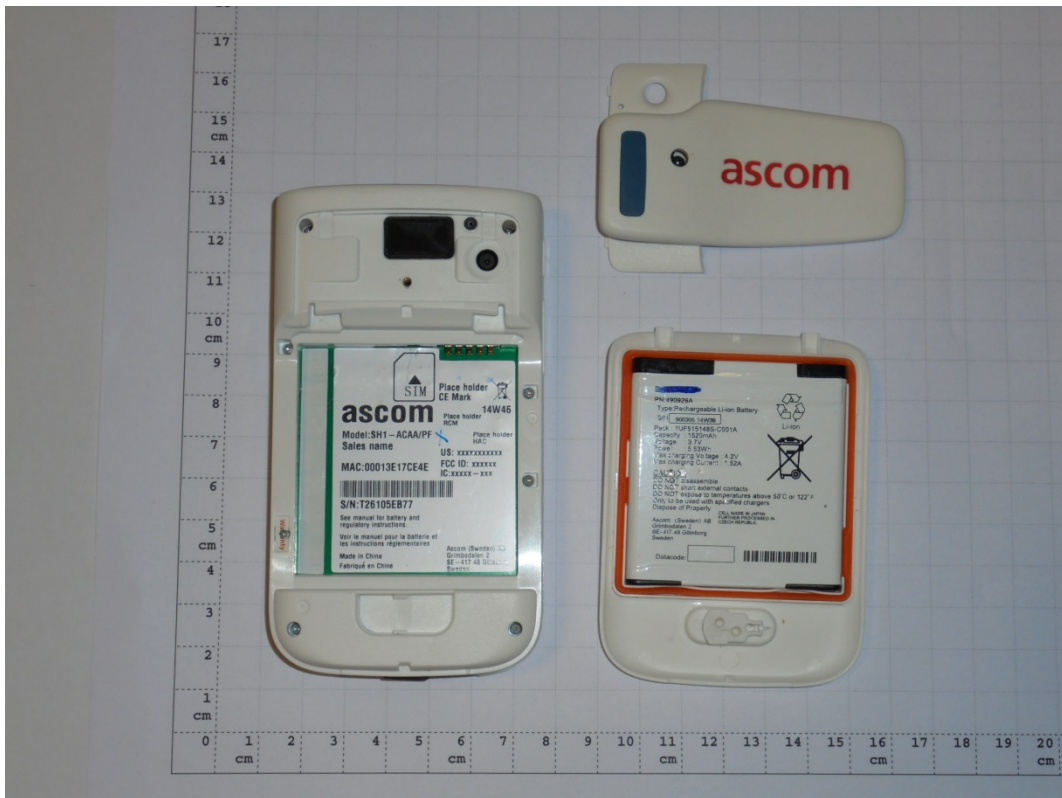
Photograph 2: EUT back side, battery and clip disassembled
