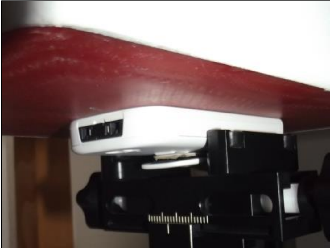
Photo 20: Test position body worn rear side with 0 mm distance
