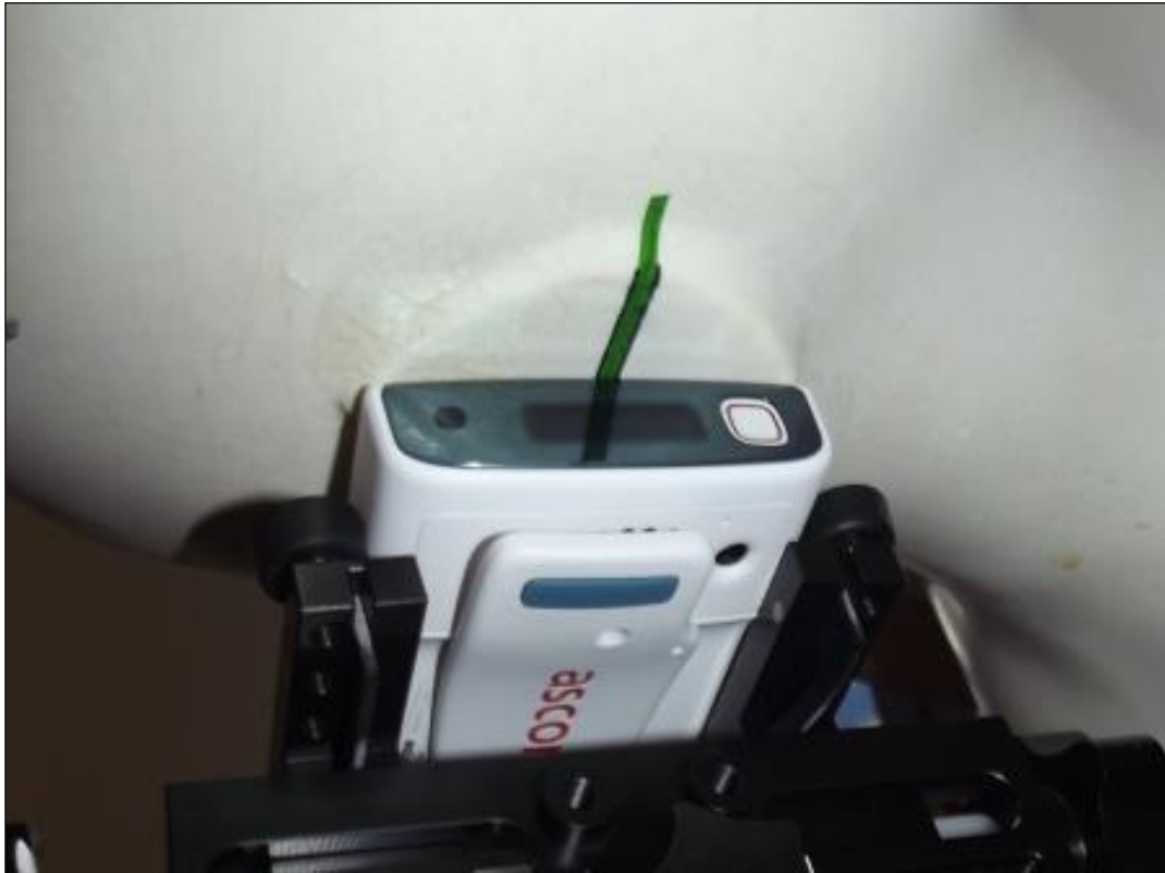
Photo 12: Test position left hand tilted 15°
