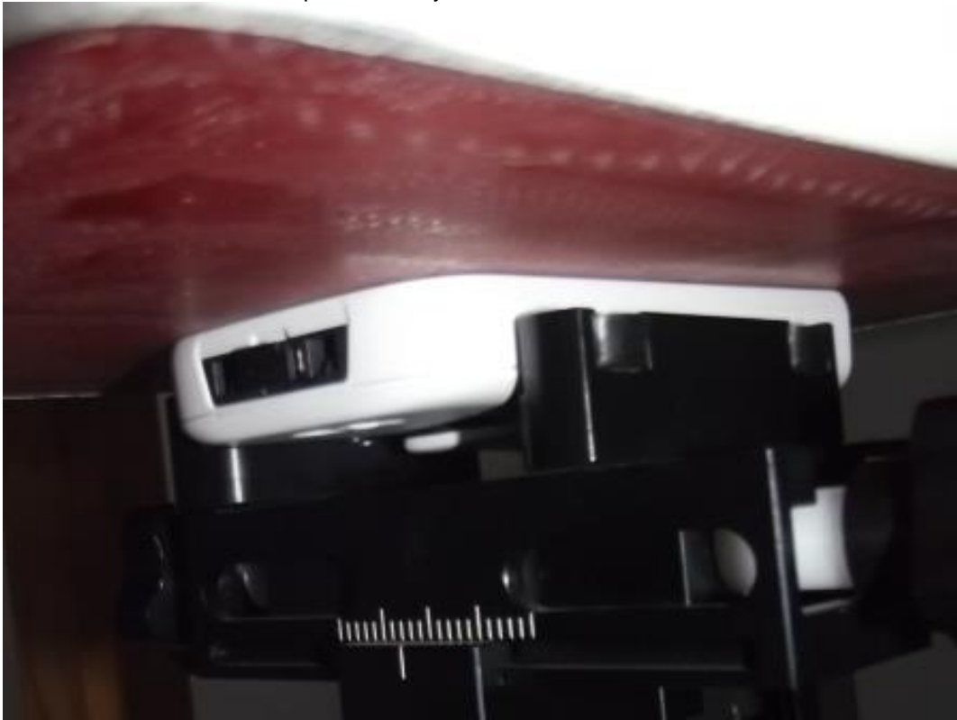
Photo 18: Test position body worn rear side with 0 mm distance
