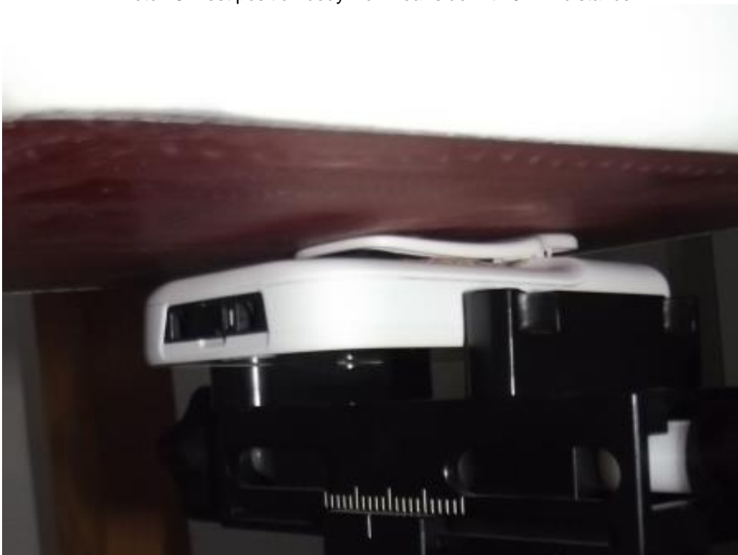
Photo 18: Test position body worn rear side with 0 mm distance
