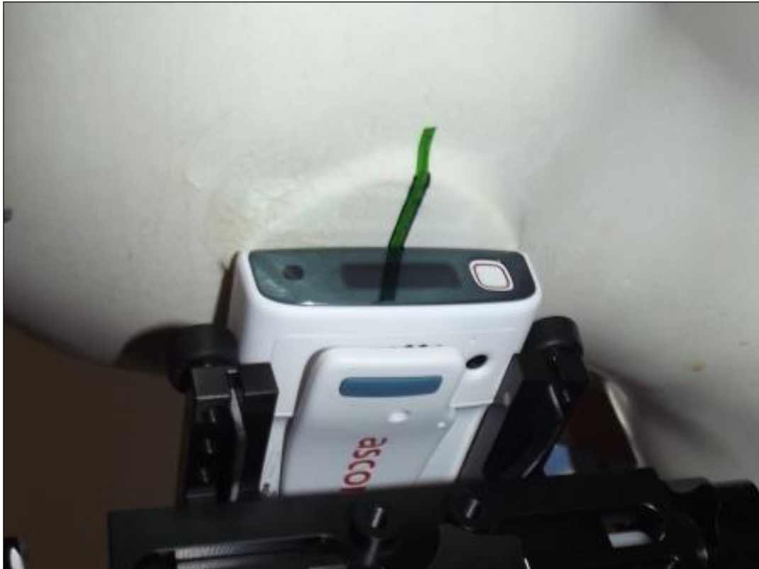
Photo 10: Test position left hand tilted 15°
