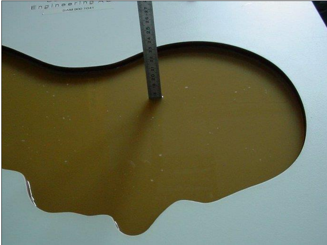
Photo 4: Liquid depth 5 GHz body simulating liquid
