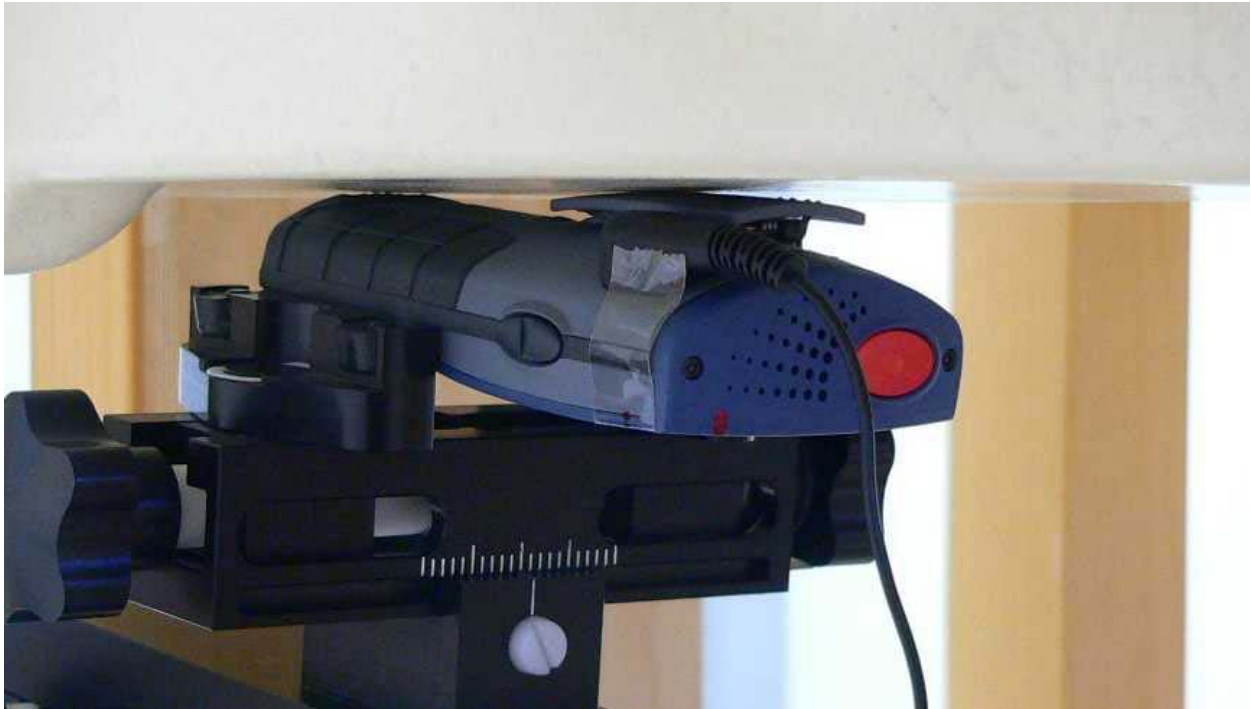
Fig. 21: Body worn, antenna 1 or antenna 2 configuration, with headset, display towards the ground.
