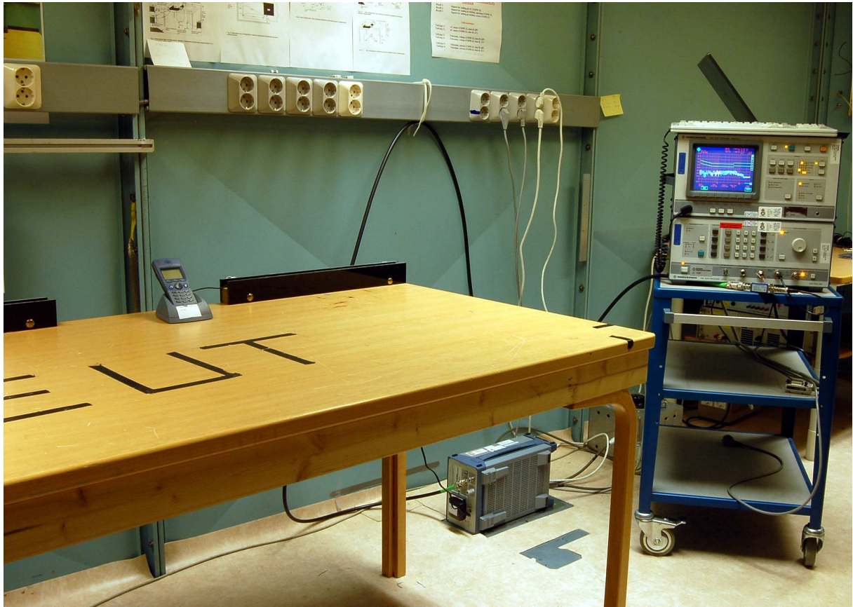
ASCOM RAID2 – Power line Conducted Emissions Test
