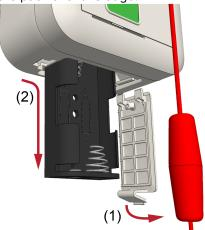
2. Place 2 x 1.5V AA disposable Alkaline batteries (not included) in the battery pack, pay attention to the polarity of the batteries.
