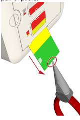
2. Insert a new button insert from the lower end of the module. Make sure the insert fits completely in the membrane.
