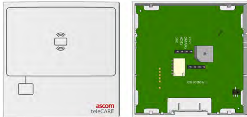
Figure 131. Card reader front and back view
