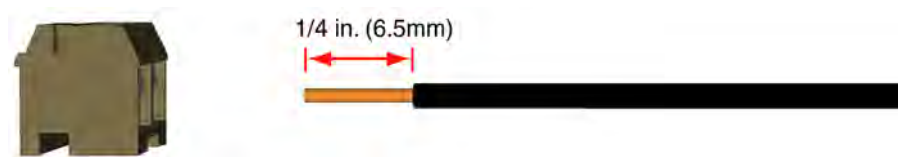
Figure 35. Stripping the wires for insertion in the connection point
