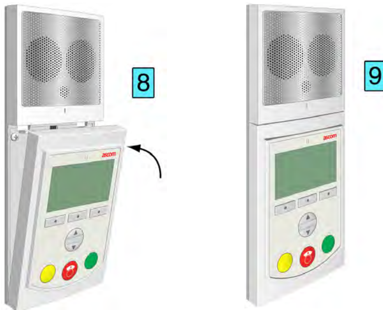
Figure 149. Mounting the NIRD on the backplate
