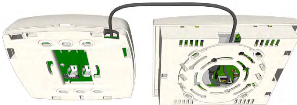
Figure 190. Example of the USB connection from NIRC3 to NUREP
