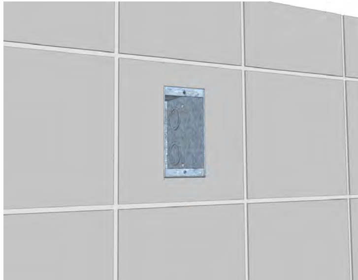
Figure 113. Positioning the back box on a tiled wall
