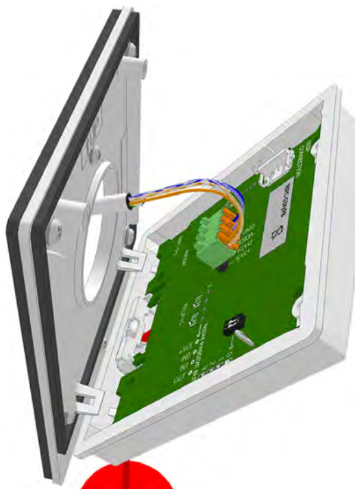
Figure 124. Connecting the room bus to the switch module
