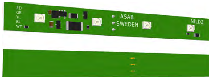
Figure 43. NILD2 - LED lamp board front and back view
