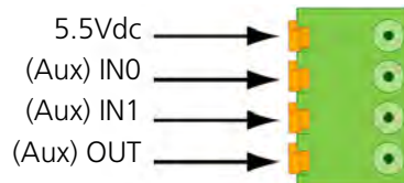
Figure 121. 4-pole connector terminal with the passive bus
