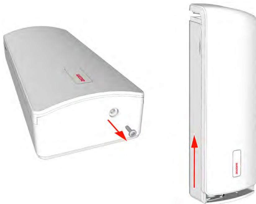
Figure 229. Removing the front cover of the NILF
