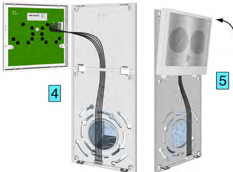
Figure 147. Connecting the NISP and mounting it on the backplate
