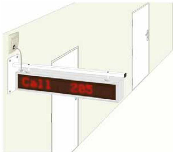
Figure 162. Wall mounted NICD
