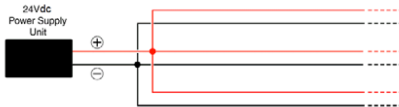
Figure 6. Multiple power buses
