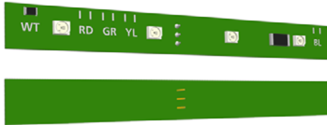
Figure 46. LED lamp board front and back view
