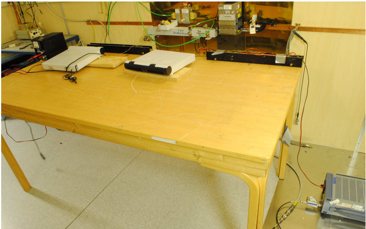
Power-line Conducted Emissions Test Set-up
