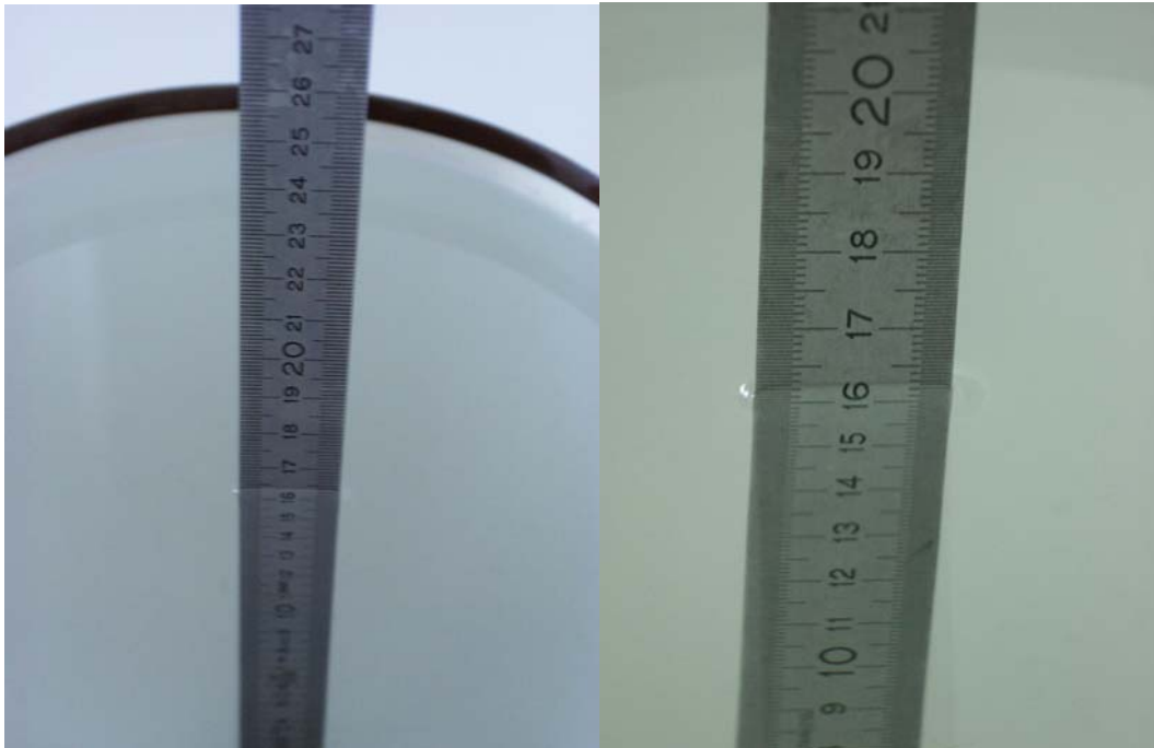
Fig. 23: Liquid depth for 2.45 GHz WLAN Head and Body measurements.
