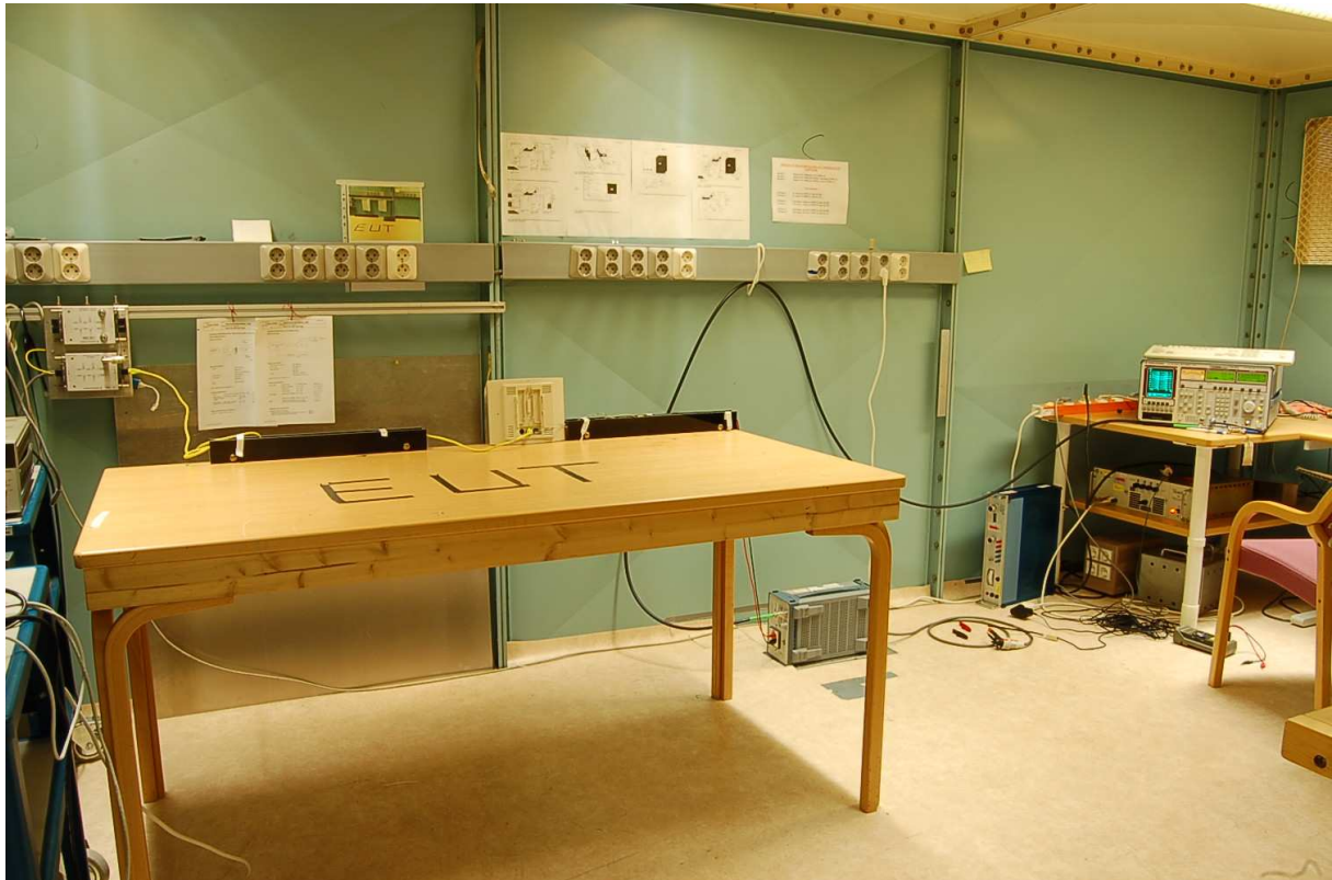
ASCOM IPBS1 – Power line Conducted Emissions Test
