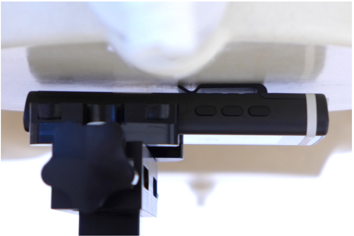
Pic. 10: Test position rear side of DUT towards the phantom, 0 mm gap, belt clip attached.
