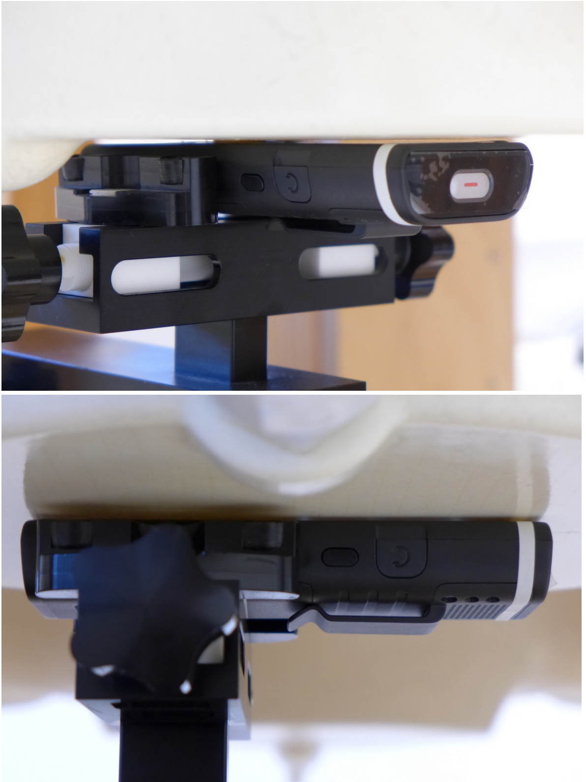
Pic. 9: Test position front side of DUT towards the phantom, 0 mm gap, belt clip attached.
