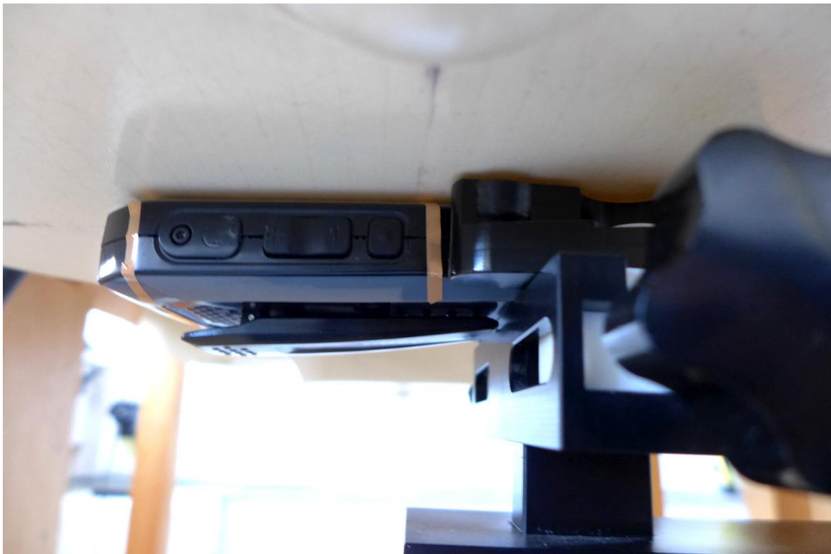
Pic. 9: Test position front side of DUT towards the phantom, 0 mm gap, belt clip attached.
