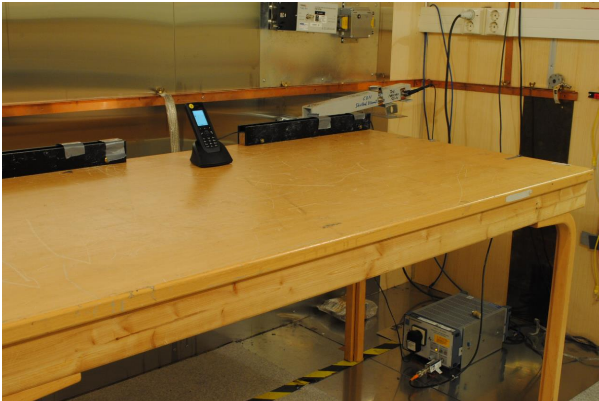
Power line Conducted Emissions Test
