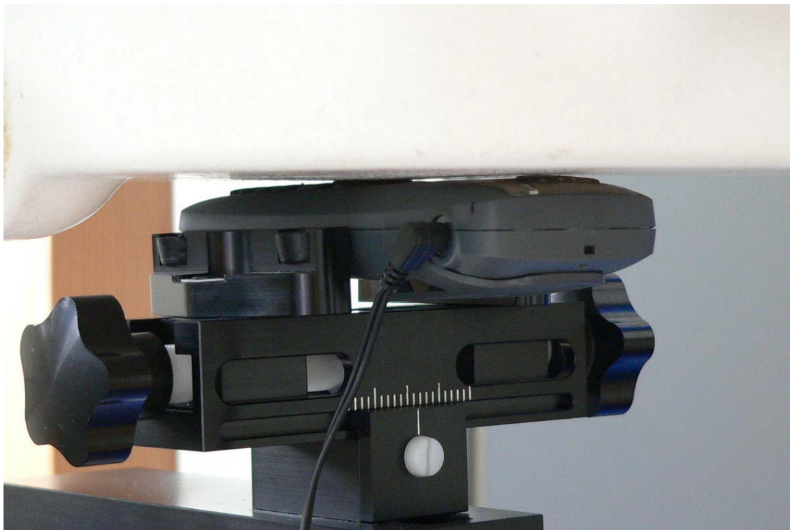
Fig. 21: Body worn, antenna 1 or antenna 2 configuration, with headset, display towards the phantom.
