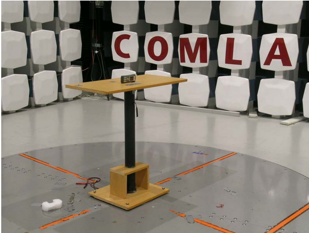
Test set-up for radiated measurements – XZ plane
