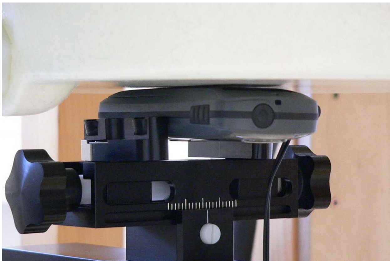
Fig. 24: Body worn, antenna 1 or antenna 2 configuration, with headset only, display towards the ground.
