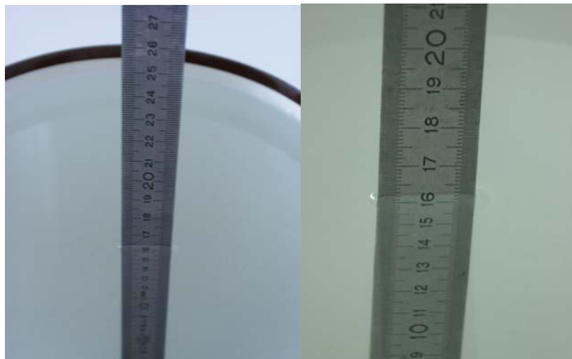
Fig. 25: Liquid depth for PCS 1900 Head and Body measurements.
