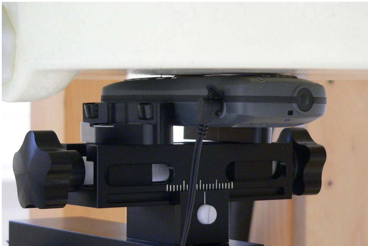
Fig. 23: Body worn, antenna 1 or antenna 2 configuration, with headset only, display towards the phantom.
