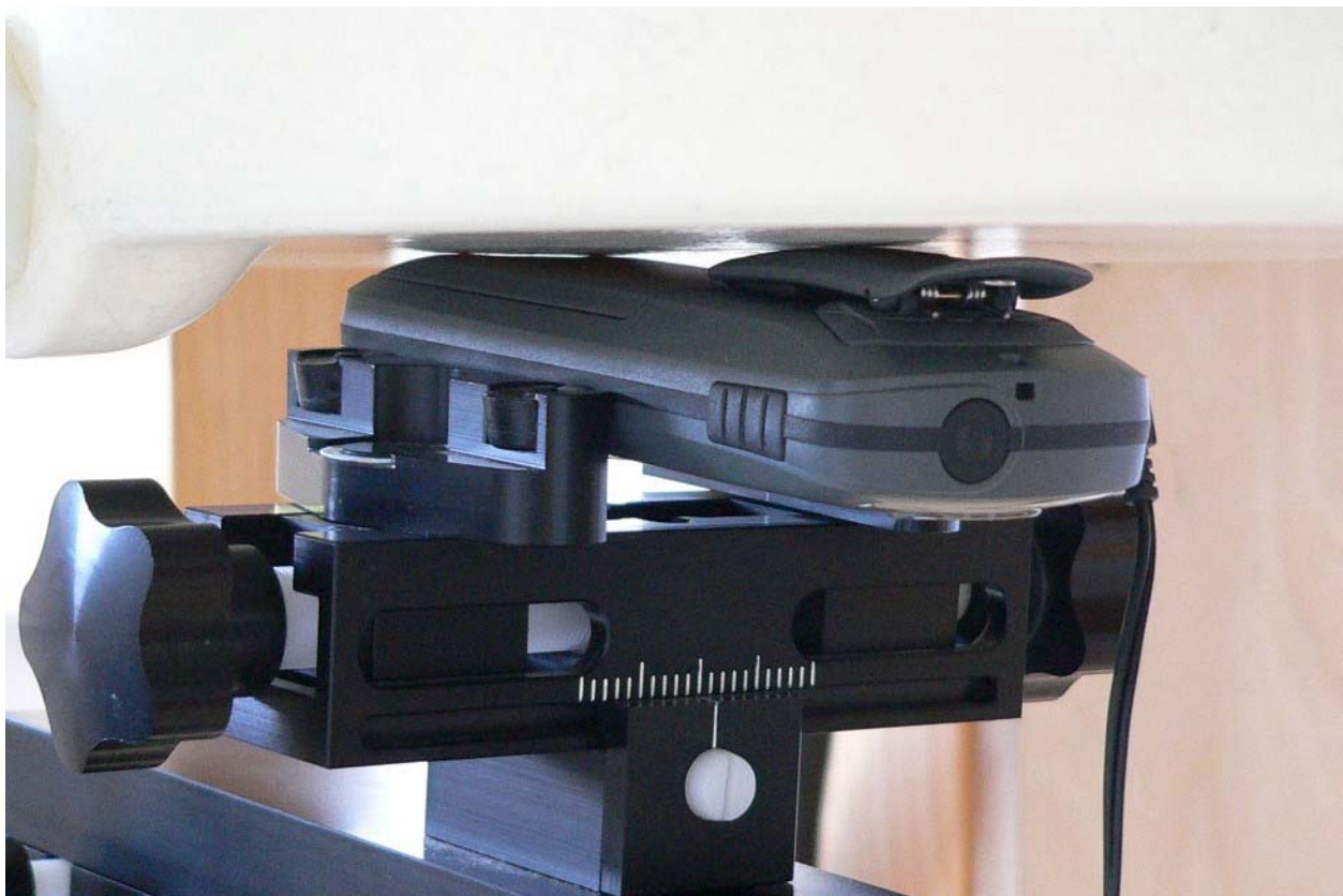
Fig. 22: Body worn, antenna 1 or antenna 2 configuration, with headset and clip, display towards the ground.
