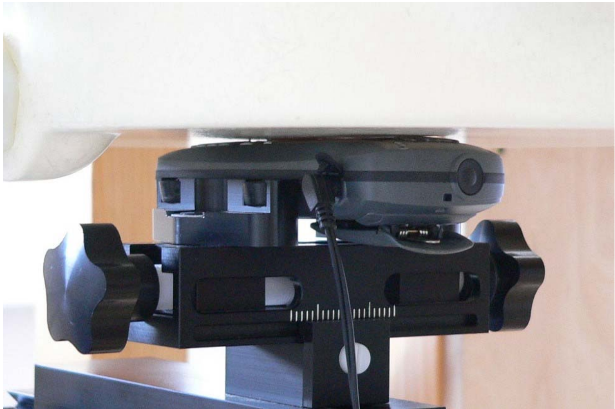
Fig. 21: Body worn, antenna 1 or antenna 2 configuration, with headset and clip, display towards the phantom.
