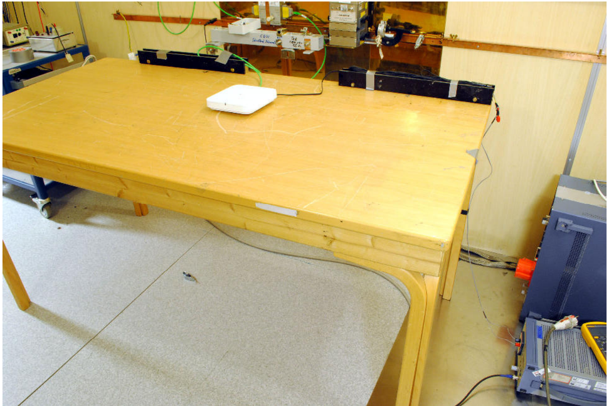
Power-line Conducted Emissions Test Set-up
