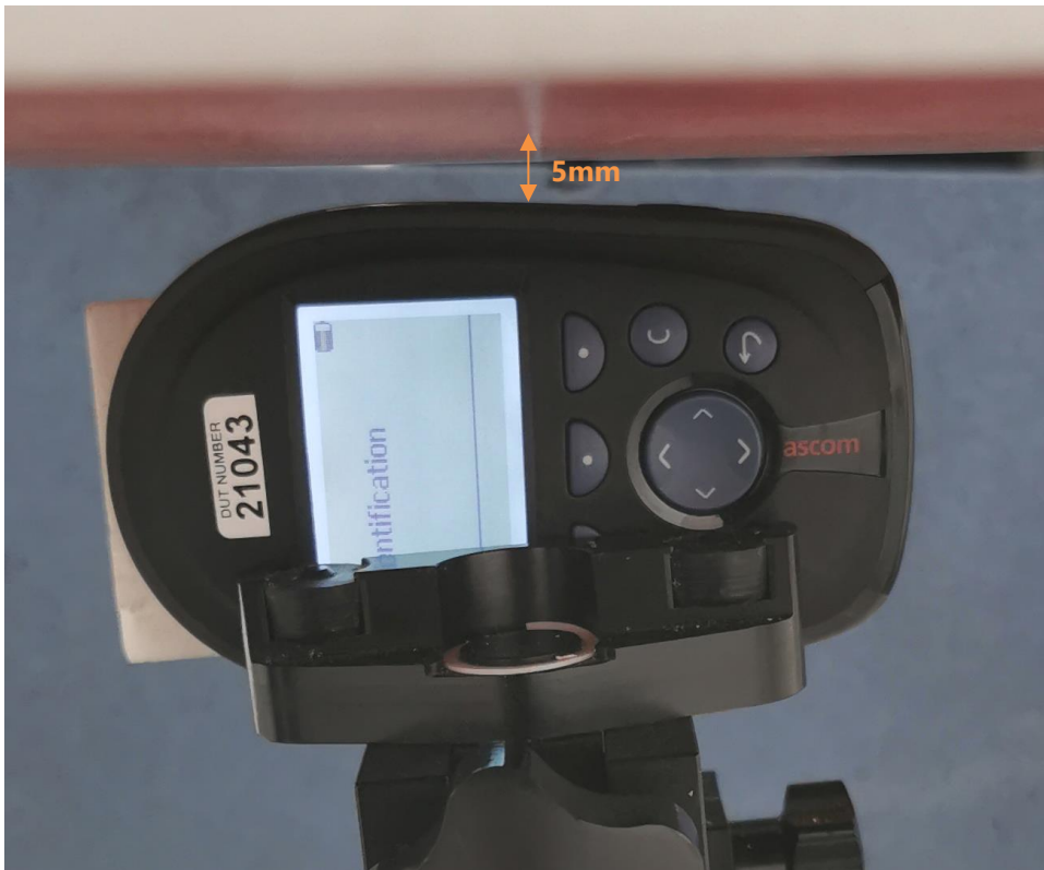
Right side of the DUT against the phantom, 5mm separation distance
