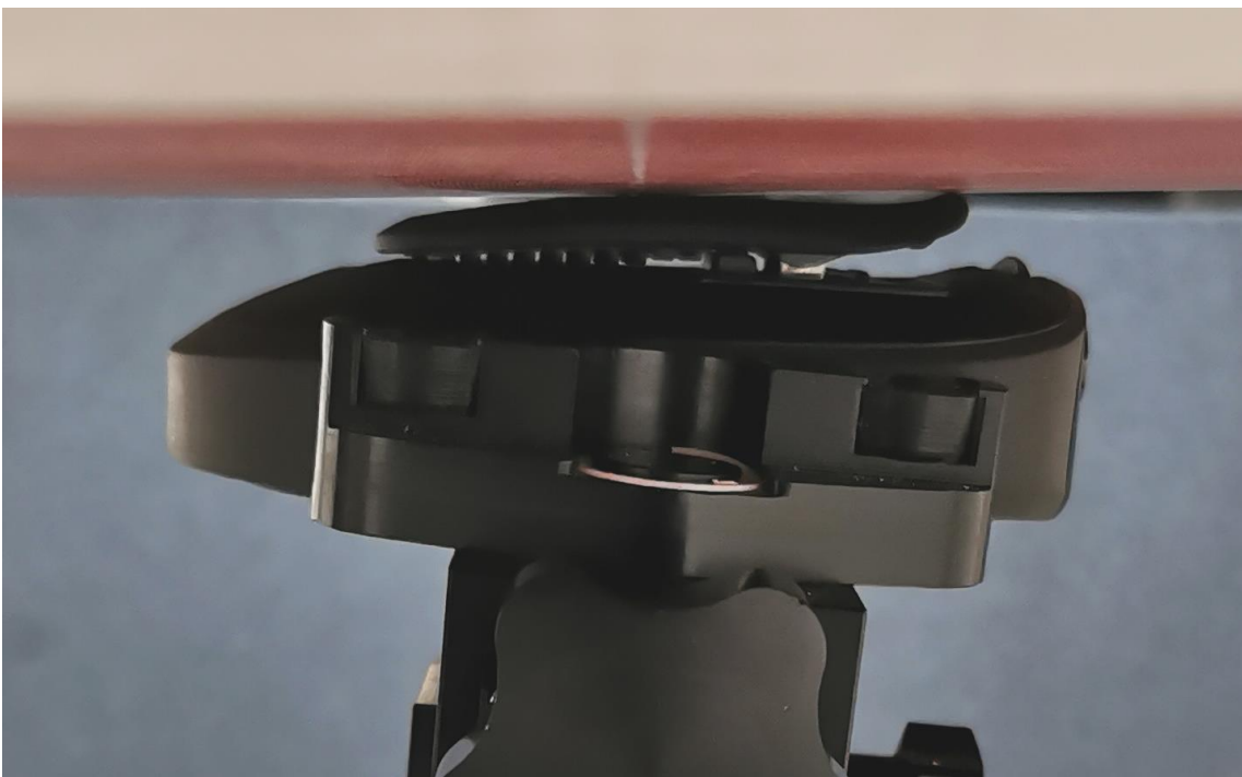
Back side of the DUT with clip against the phantom, 0mm separation distance
