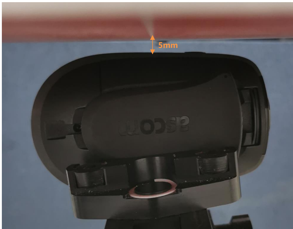
Left side of the DUT against the phantom, 5mm separation distance
