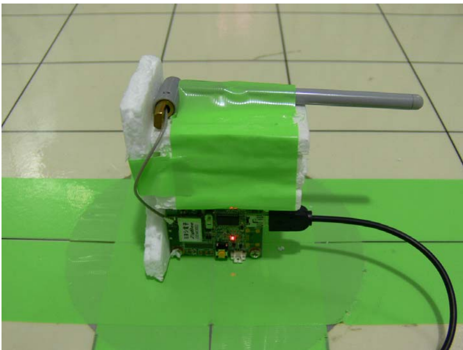
Photograph 13: Set-up for Radiated Emission, EUT Configuration external antenna Y-Axis
