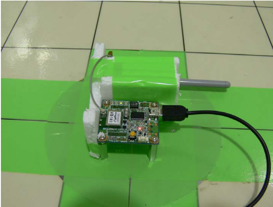
Photograph 12: Set-up for Radiated Emission, EUT Configuration external antenna X-Axis
