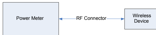
Figure 5-1 Power Measurement Setup
