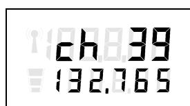
**EXAMPLE:** Channel memory number »39« (with the channel name 132.765) should be deleted.
