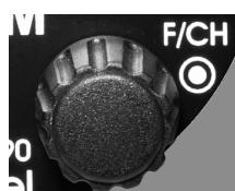
Rotary control and push-button = dual function
