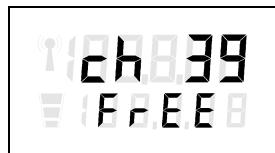
If this channel memory should really be deleted confirm by pressing the **STO** button. In the lower line the frequency/channel name disappears, it appears »FREE«.
