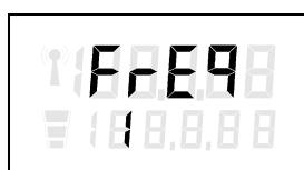
The display shows in the upper line alternately »SET« and »FREQ«, in the lower line »0« or »1«.
