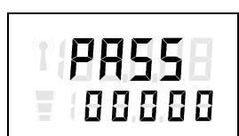
The display shows in the upper line alternately »SET« and »PASS«, in the lower line »00000«.
