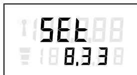
»8.33« = combined 8.33 and 25 kHz channel spacing.
