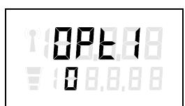
The display shows in the upper line alternately »SET« and »OPTI«, in the lower line »0«.
