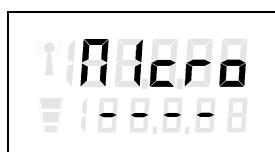
The display shows in the upper line alternately »SET« and »MICRO«.
