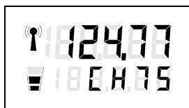
Transceiver operates in the '**25 kHz only' mode (5-digit display)**
