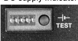
LED indicator to check the capacity of the built-in battery or external DC supply.
