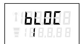
The display shows in the upper line alternately »SET« and »BLOC«, in the lower line »0« or »1«.
