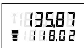
Transceiver operates in the '**25 kHz only**' mode
