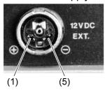
2-pole twist-lock socket to supply the radio by external 12 Vdc sources.
