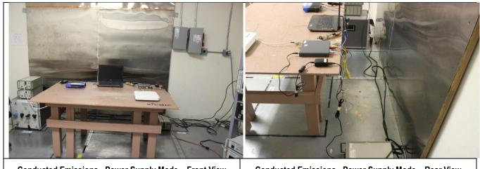
Conducted Emissions - Power Supply Mode - Front View
