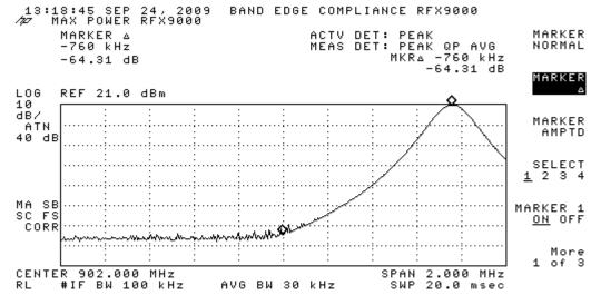
High side, non-hopping and hopping respectively. Band edge is 928 MHz; emissions are more than 30 dB below the in band signal.
