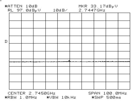
No higher harmonics or other emissions found in either vertical or horizontal in the chamber.
