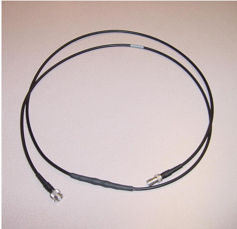
Photo of Shorter Cable Assembly with Attenuator
