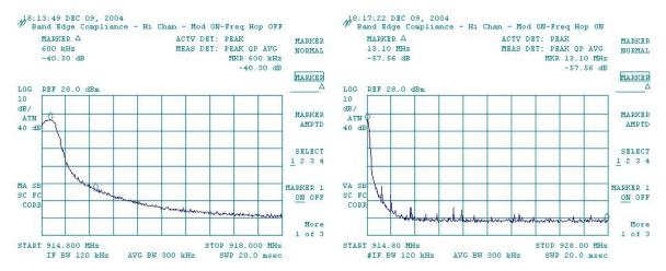
High side, non-hopping and hopping respectively. Band edge is 902 MHz; emissions are more than 30 dB below the inband signal.
