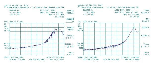
Low side, non-hopping and hopping respectively. Band edge is 902 MHz; emissions are more than 30 dB below the inband signal.
