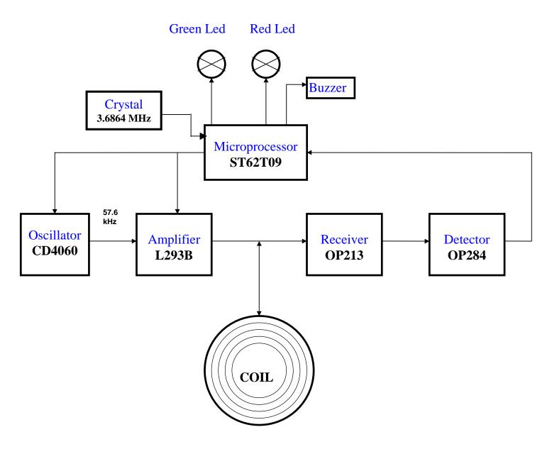
The oscillator generate a tension of which frequency is about 58 kHz.
