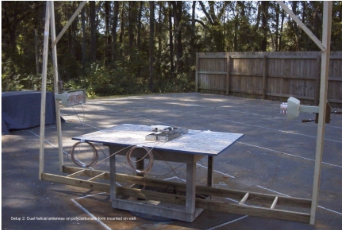
Setup #2: Dual helical antennas wound on polycarbonate forms in wall mounted assemblies.
