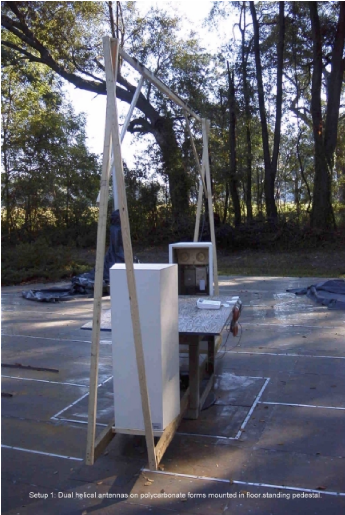
Setup #1 Dual helical antennas wound on polycarbonate forms in floor standing kiosk.
