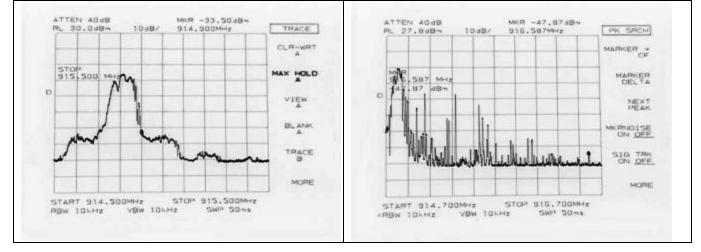
Low side, non-hopping and hopping respectively. Band edge is 902 MHz; emissions are more than 40 dB below the inband signal.
