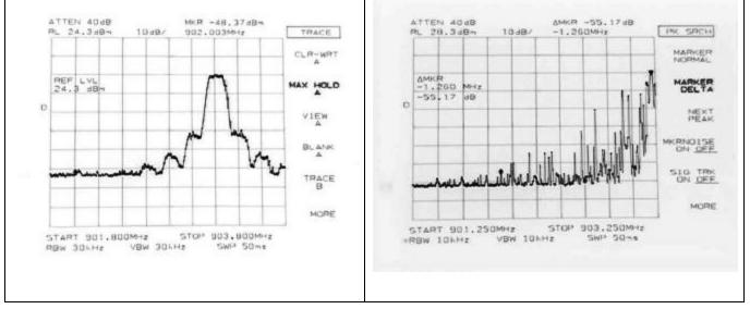
The following 2 plots shows that there are no emissions within 20 dB of the inband signal in any 100 kHz band all the way to the  $10^{th}$  harmonic.
