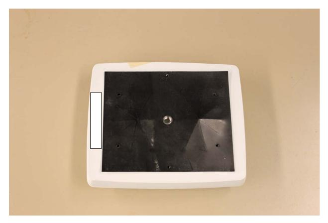
One FCC/IC label will be placed in the position indicated. This is an outside surface.
