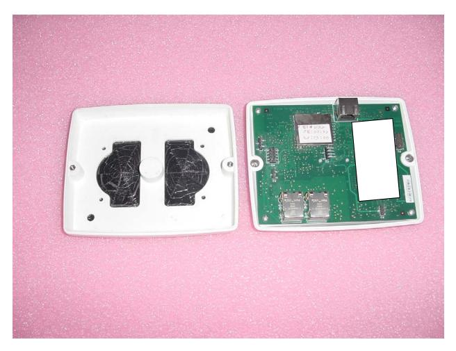
One Regulatory label (white rectangle in photo) will be attached to PCB. This is visible during installation.
