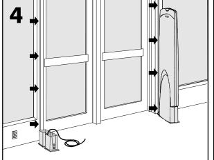
Peel and stick wireway is provided. The cable from the secondary pedestal to the primary pedestal runs up, over and down the doorway through this wireway.
