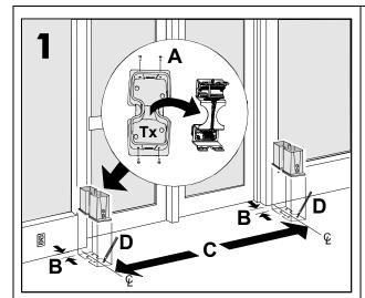
The APS-1000 uses a primary pedestal and a secondary pedestal (the one with the long cable attached).
