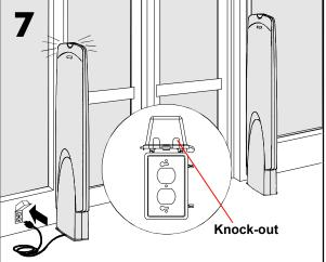
Remove the cord access knockout from the bottom of the ac receptacle guard (supplied). Replace the existing outlet cover with the receptacle guard.
