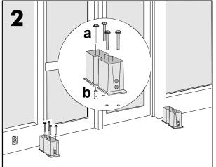
Secure each base using screws (a) and anchors (b) supplied.
