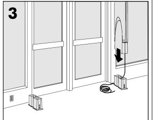
With its bottom facing the doorway, gently lay the secondary pedestal near its base. In the base, run the cable through the Romex clamp in the lower hole facing the door. Tighten the Romex clamp.
