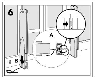
A. Gently lay the primary pedestal near the base with its bottom facing the doorway.
