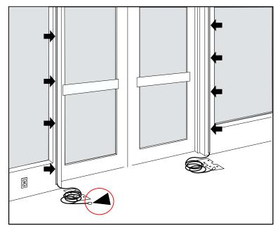
• If you are trenching the floor between the pedestals, ensure the proposed trench extends under the pedestal location so cables can enter the pedestal from its base underneath. Then, using a floor saw, trench the floor from pedestal to pedestal. The depth of the trench is 1 centimeter, or 3/8 inches. The width of the trench is 1 centimeter, or 3/8 inches.
