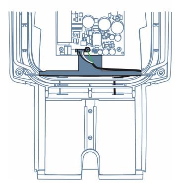
**WARNING:** Do not run the power and comm cables in the same conduit or raceway. Building codes require that power wiring be separated from other types of wiring.
