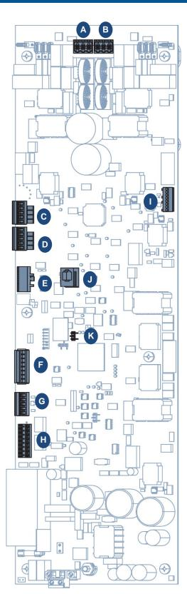
\* Connect RS-485 options by connecting the RS 485 LO wire to the RS 485 LO pin and the RS 485 HI wire to the RS 485 HI pin. \*\*To override the normal boot process, short pins 1 and 2 of connector P18.
