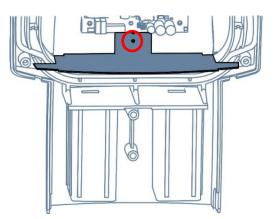
5. Loosen the ground screw, positioned to the right of the power connector. For the location of the ground screw, see **Figure 10**.
