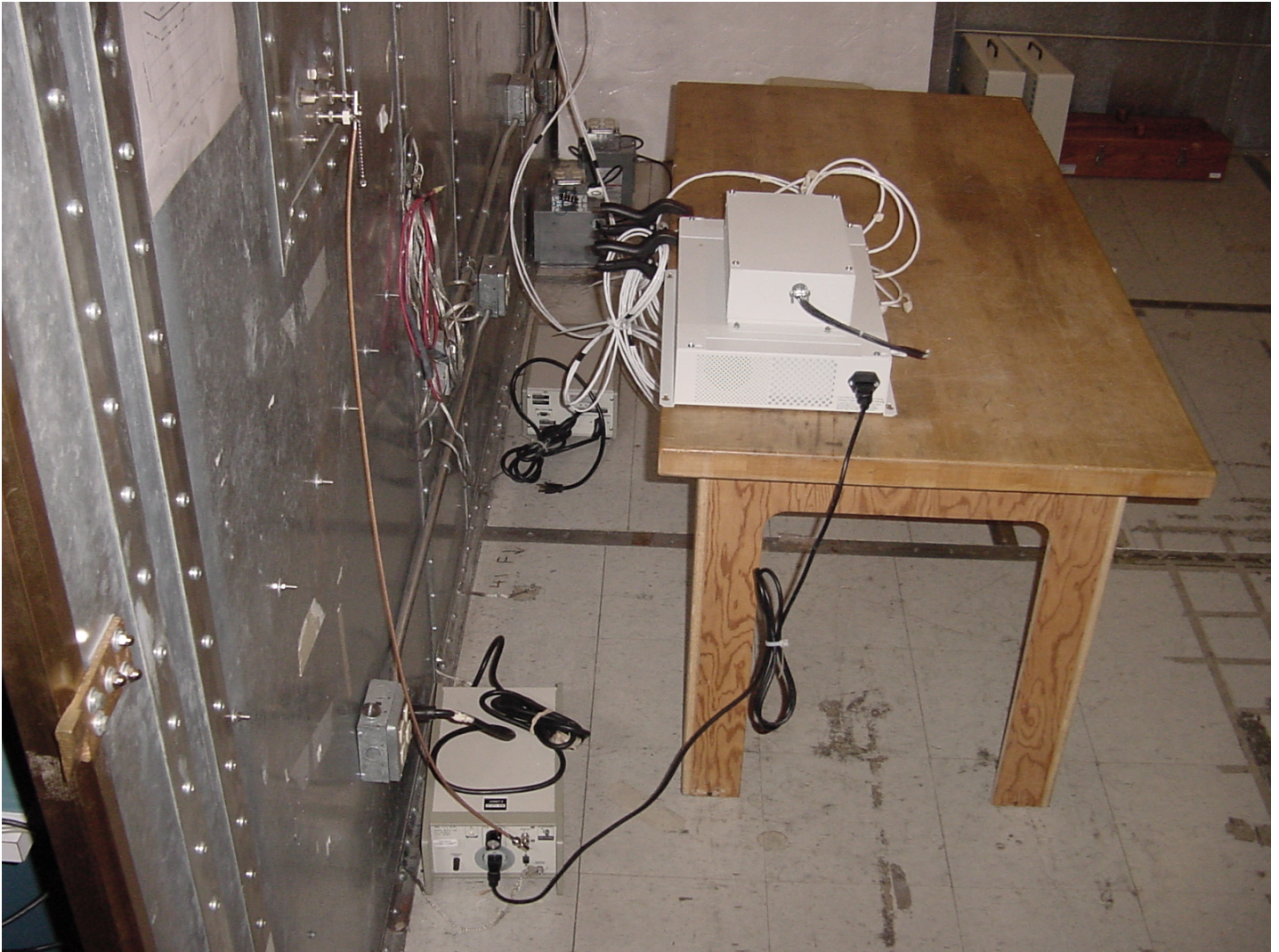
DUT on left corner of table, accessory layout, antenna cables routed to exit chamber through waveguide. With AMC-7000 metal detection option on top
