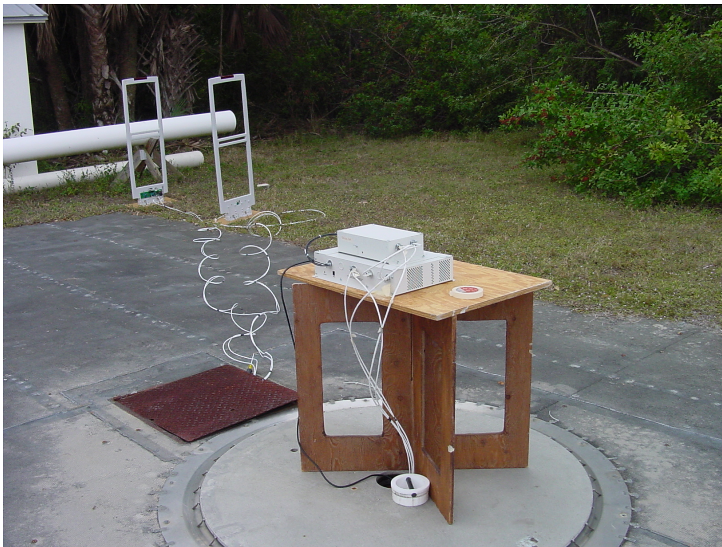
Radiated Emissions over 30 MHz.at OATS
