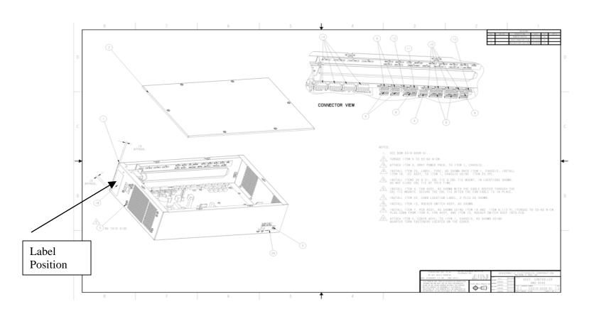
The label is a metalized polyester that is UL recognized and is permanently affixed using an L-23 adhesive.
