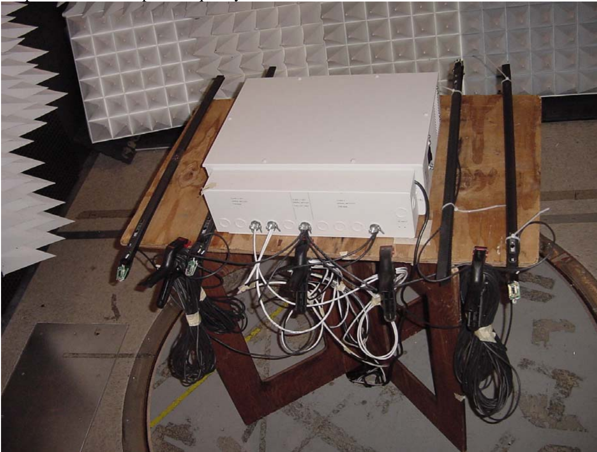
3 meter compact chamber setup for frequency identification
