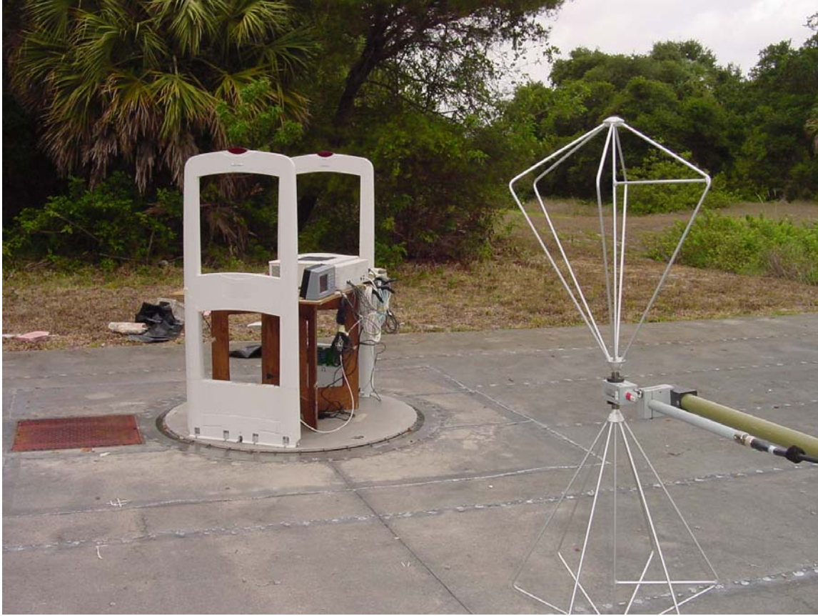
Typical OATS setup. Alternate antenna used for rotating system.
