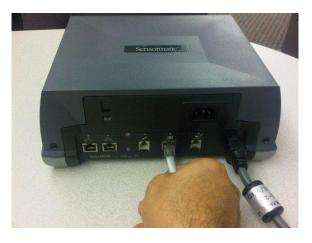
3. Plug the AC power cord into the power supply and its other end into an unswitched AC outlet having less than 0.5Vac between neutral and ground. The Status LED should be solid green. Note: While the controller auto-synchronizes, the Status LED may briefly flash amber. Autosync can take up to ten seconds.
