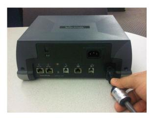
Plug the barcode scanner interface cable (if used) into the scanner port of the controller.
