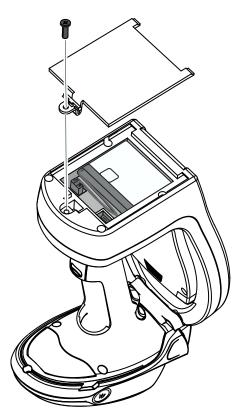
2. Remove the battery and disconnect it.
