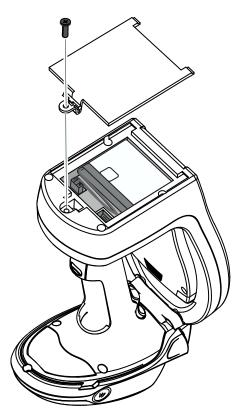
2. Remove the battery and disconnect it.
