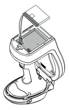
3. Plug in the new battery, bend wires as shown, and seat it in the battery compartment. Install the battery cover and secure it with the screw. DO NOT over tighten.
