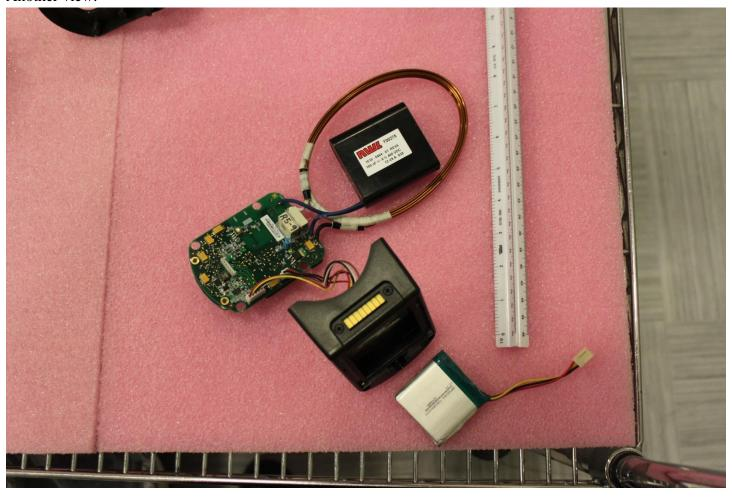
Co-planar boards. Digital, power, deactivator board showing. Reverse side shown below.
