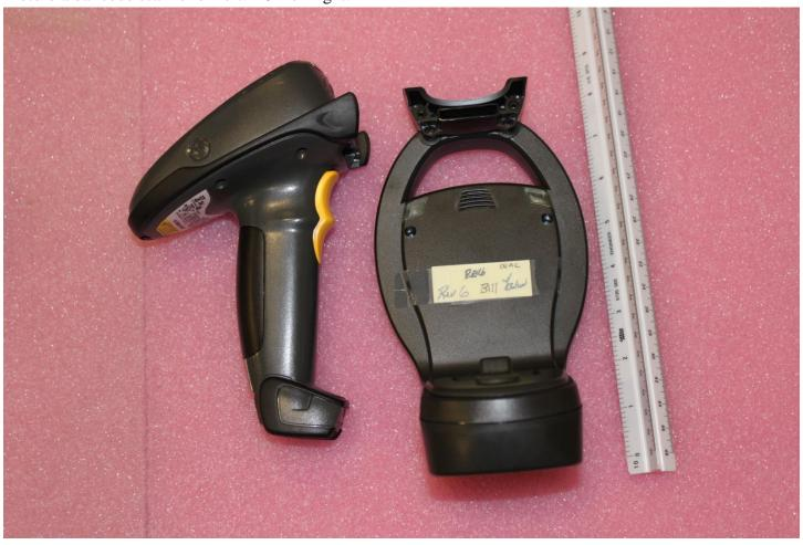
Battery fits into base. Contacts are for charging and communications with bar code scanner. FCC label to be applied inside battery compartment.
